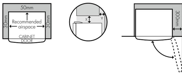
*NOTE: Refrigerator doors on all models are designed to sit proud of cabinetry (not flush). The refrigerator should be placed against a wall of cabinetry and the clearance between the rear of the refrigerator and the wall should not be greater than 75mm.*
