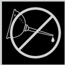
The motor is permanently lubricated and requires no oiling. Because your Air Circulator moves a substantial amount of air, it will need regular cleaning. Unplug the unit before any cleaning activity.
