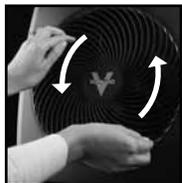
**Models V102, 270** • Remove the screw located at the 6 o'clock position. Rotate the grill counter-clockwise to unlock and then lift off. To reinstall the grill, position the grill with the logo slightly turned to the left and rotate clockwise. Replace the screw.
