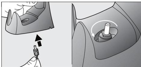
Seat the handheld vacuum on the wall mount bracket, the vacuum can start charging in this position.
